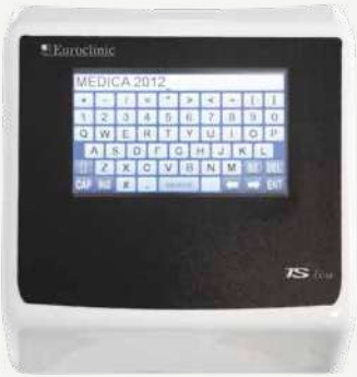
Color and orientable touch screen display on instruments tablet, with articulated arm, for instruments control.
