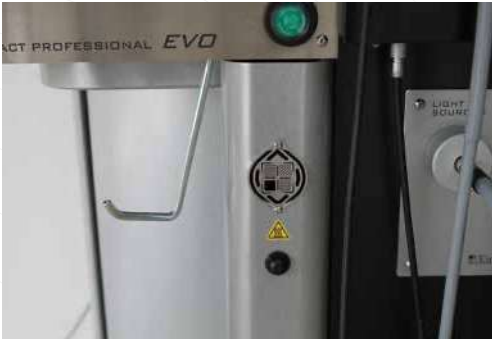
Mirror warmer with time setting by touch screen (10-120 sec).
